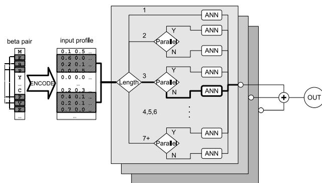
Fig. 4. The BCEval architecture. The guarding functions ensure that only one neural network is activated at a time. The “parallel” guard is able to distinguish between parallel and anti-parallel strand pairs, while the “length” guard dispatches based on the length. In the example, an anti-parallel pair of length 3 is given so activating the path shown in bold. Three core units consisting of independently trained neural networks are averaged to obtain the final evaluation.
